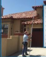
Our inspectors use the Spectoscope, a tall telescoping pole camera which allows them to safely take high quality pictures of the roof, hard to get to roofs, chimneys, skylights and other areas of a home from the ground.
